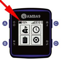
Hold button A to power on. Check the main screen to see if the unit is fully charged. "100%" will display in top left corner of screen.
