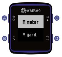
Press button C or D to select "Y yard" and press button A.
