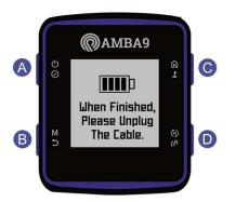
Scroll to gear icon by pressing button C or D to acces the Setting menu. Press button A.
